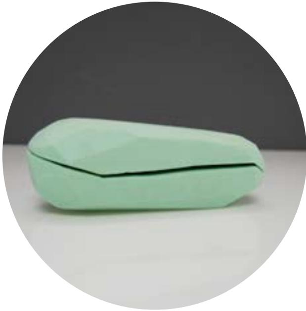
CNC model no.1 (finally!) of the final idea. This model allowed more thought towards designing the way the cables fitted in.
