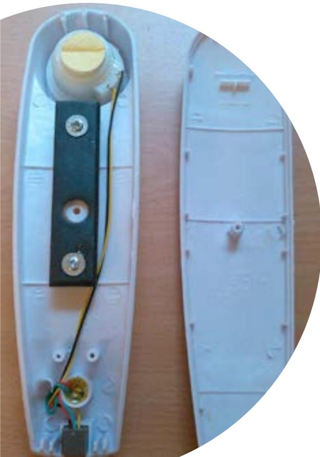
The components appear to be bought in, forcing the phone to be designed around the parts. Bosses and ribs have been designed into the mouldings to aid structural strength to the casing and to provide spacing and positioning of the parts with minimal fixings - reducing the overall cost, too.
