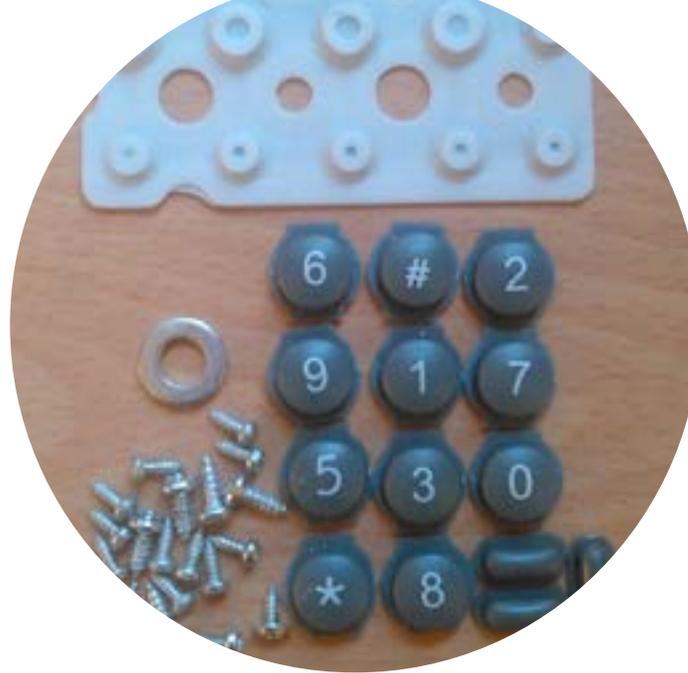
The numbers on the buttons may have been tampon printed. As it is CNC-controlled, it's quick and efficient, thus making it a cheap and sustainable method.
