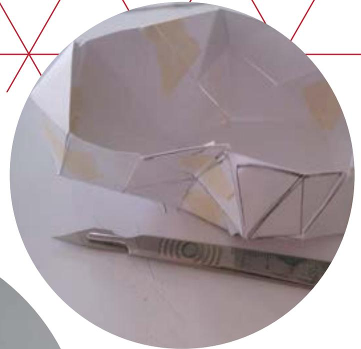
Testing a combination of paper folding and tessellations - unsuccessfully. The model was weak, lacking in aesthetic form and difficult to manipulate.
