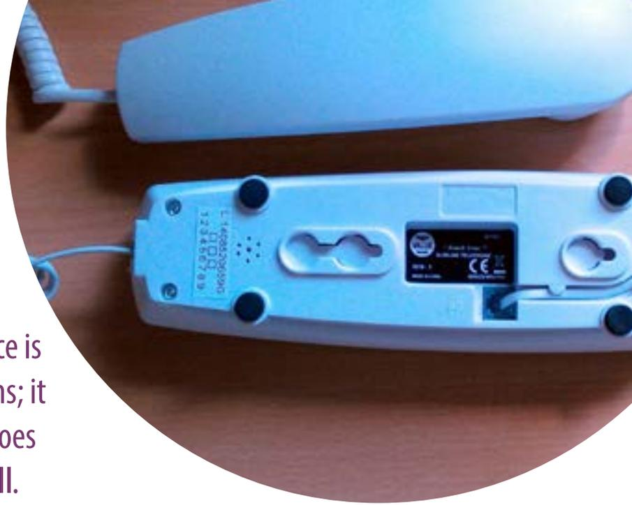
The body is made of white injection-moulded spark finished ABS and the same in grey for the buttons, as suggested by the ejector pin marks (unburred) and recycling symbol in side the handset.
