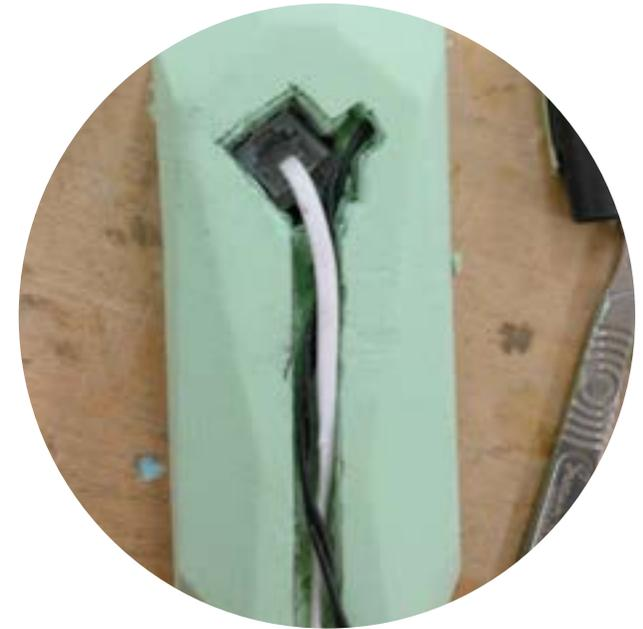
Deeper channel and moulded-in spaced for the telephone cable and mains cable (to be made so it is fitted. Removability would be unnecessary on a small appliance such as this).
